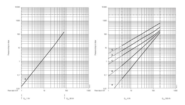
Viscosity diagrams: A = 5 mPa.s C = 100 mPa.s E = 500 mPa.s D = 200 mPa.s
