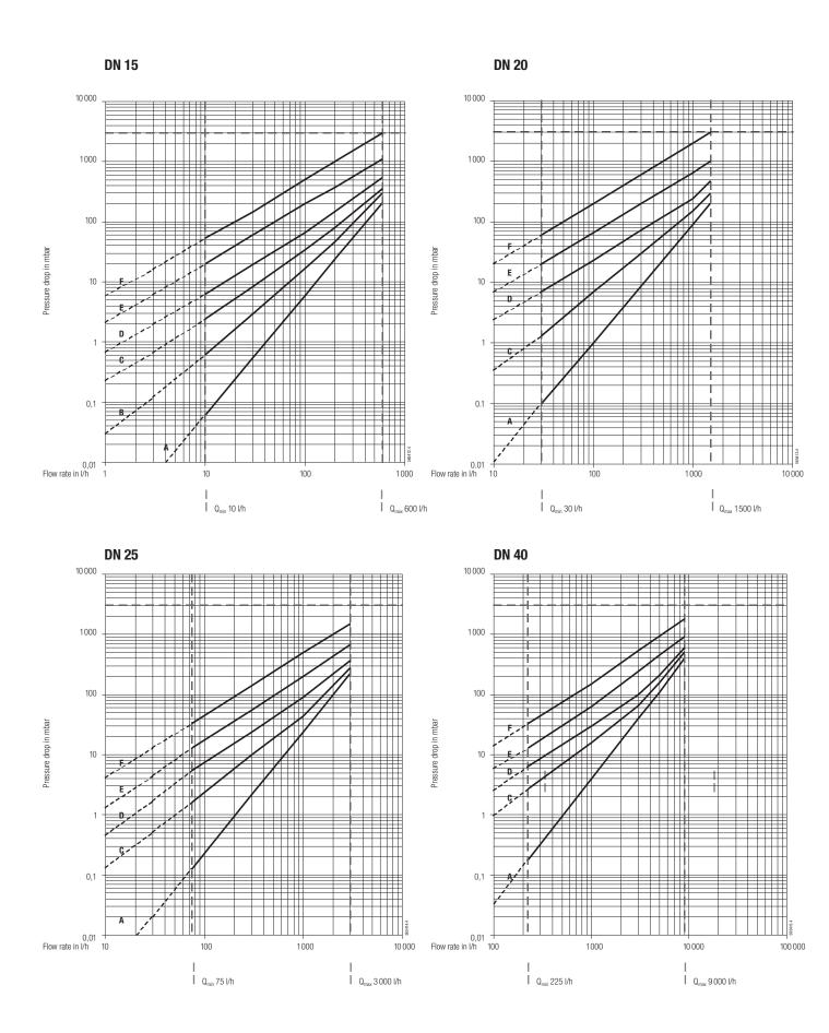
For a pressure drop of more than 1 bar, it is recommended to use the next larger meter size. Maximum permissible pressure drop = 3 bar
