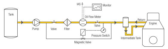
Float or valve control in the intermediate tank is required. Formation of gas is to be avoided. The magnetic valve opens as soon as the pressure drops below a defined level. For measuring the consumption of more than one engine, each will require a separate installation similar to the one above.
