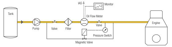
The magnetic valve opens as soon as the pressure drops below a defined level.
